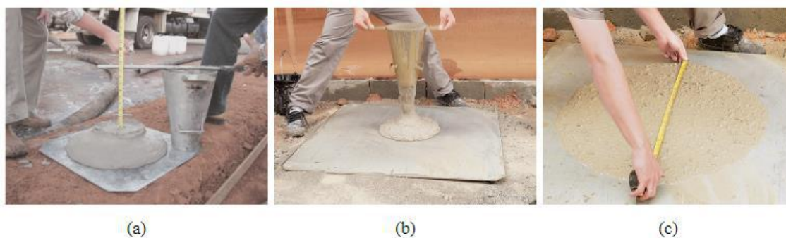
Figura 2.3 – (a) Slump test; (b) e (c) Slump flow test.
