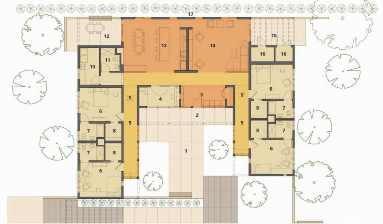
TYPICAL RESIDENCE FLOOR PLAN 1 ENTRY COURT 2 PORCH 3 ENTRY 4 STAFF OFFICE 5 HALL 6 BEDROOM 7 BATHROOM 8 CLOSET 9 SKYLIGHT ABOVE 10 LAUNDRY ROOM 11 STAFF BATHROOM 12 DINING TERRACE 13 KITCHEN | DINING ROOM 14 LIVING ROOM 15 TERRACE 16 UTILITY ROOM 17 BIO-SWALE
