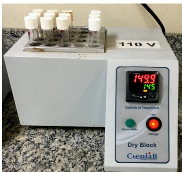
Figura 8 – Digestora Dry Block.
