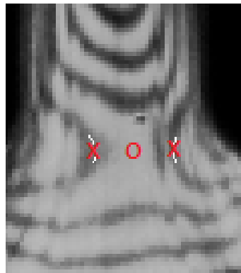
Figure 6.23: Example of the detection of the inflection point. The center of the white contours associated to each vertical fringe is marked as a cross and the estimated inflection point is marked as a circle.
