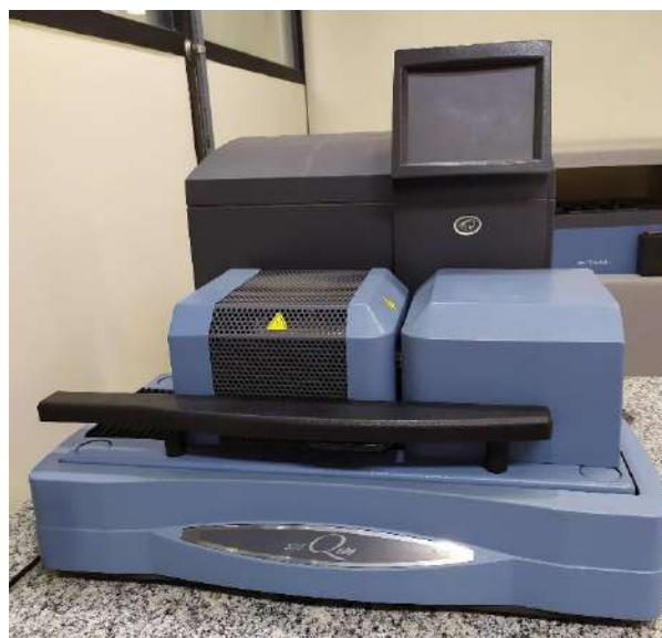
Figura IV.8 – TG/DSC SDT Q 600 da TA Instruments.
