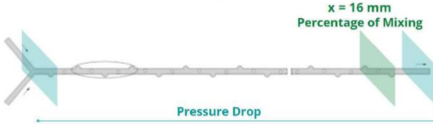
Figure 3.7: Measurements to calculate pressure drop ( x = 0mm and x = 20mm ) and blend percentage ( x = 16mm ).
