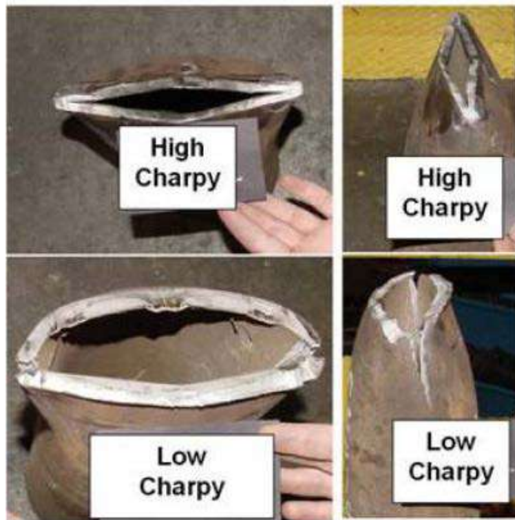
Figure 3.8: Fracture morphology of two drill pipe with different Charpy impact values[15]
