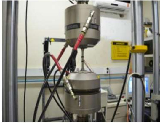
(a) Uniaxial tension test setup
