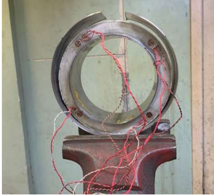
Figure 5.14: The state of CFS-A after cutting
