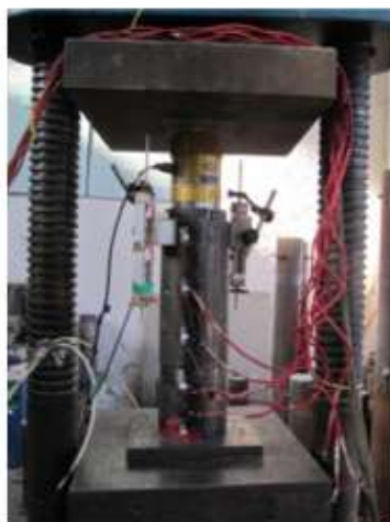
Figure 2.6: Push-out test arrangement by Lu [51]
