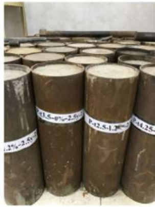
(a) CFST columns with concrete core
