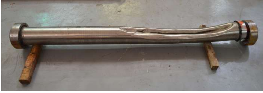
Figure 4.6: Tested SP1 sandwich pipe
