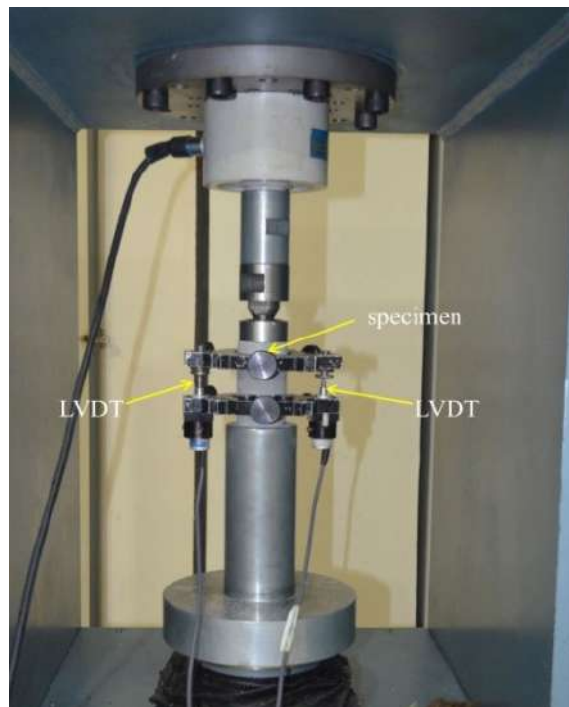
Figure 3.2: Uniaxial compressive test set up
