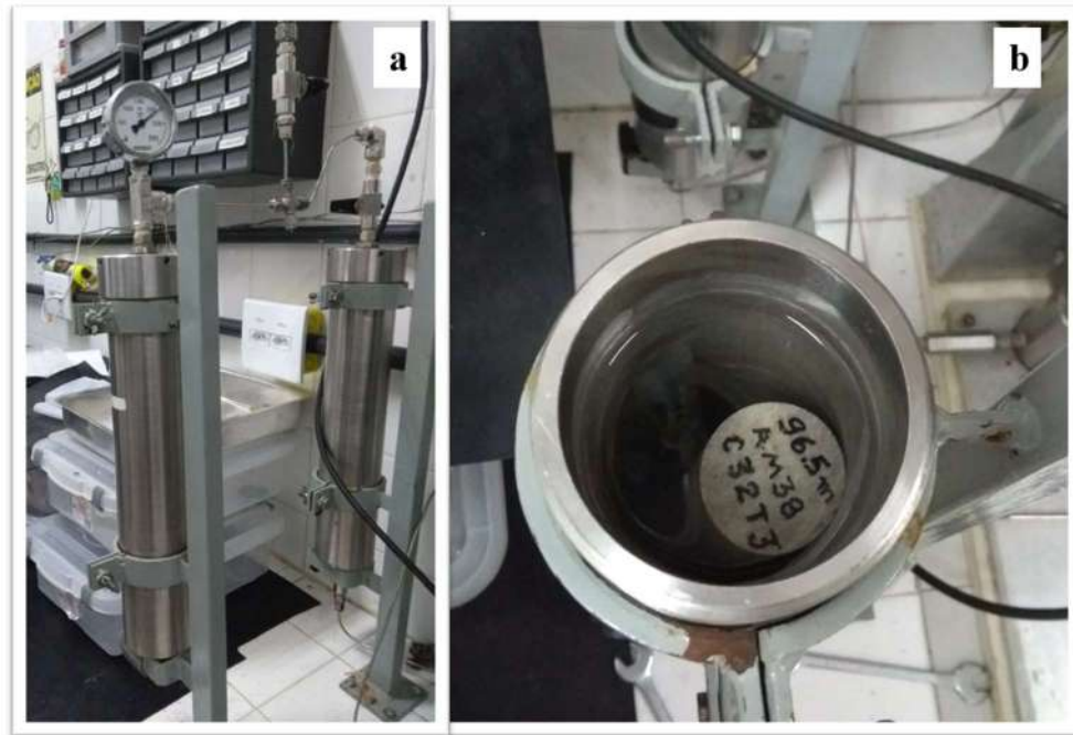
Figure 3-2 - Photo illustrating saturation of low permeability samples. a) Cell where samples remained for 24 hours, immersed in brine and under the pressure of 2,000 psi; b) Detail of the interior of the cell containing a sample immersed in the fluid
