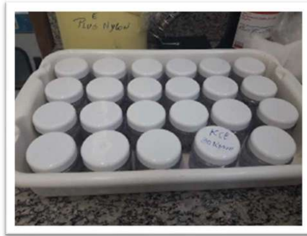
Figure 3-3 - Samples stored in brine-filled containers to maintain saturation for NMR analysis
