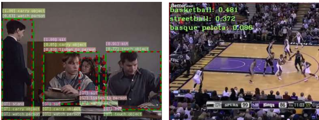
Figure 1.1: Output frames from action recognition systems that perform localization and classification of actions in video. Source: [12, 19]
