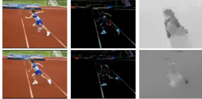
Figure 2.3: Comparison between the three different types of input data: RGB (left), RGB difference (center) and optical flow vectors (right). Source: [31].
