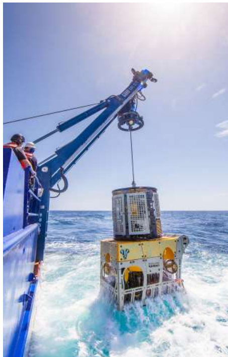
Figure 1.1: ROV being deployed - source: www.technipfmc.com
