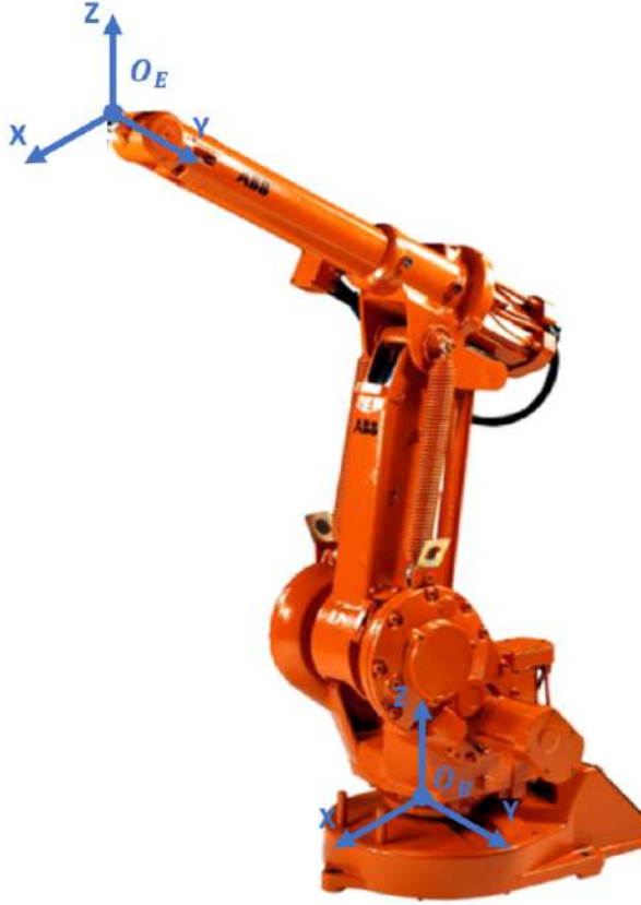
Figure 2.1: Manipulator with base and end-effector coordinate systems. This image is modified from https://new.abb.com
