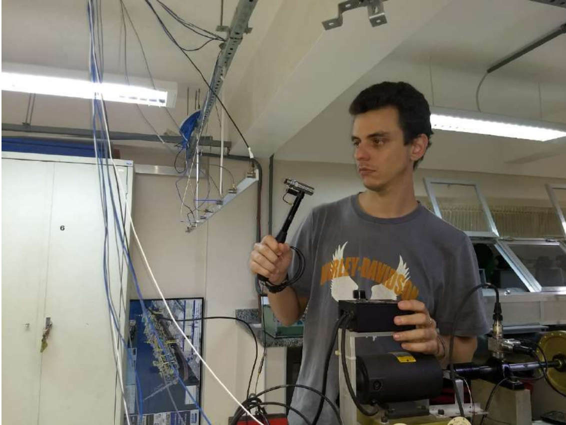
Figure 5.5: Aluminum beam being excited by impact hammer.
