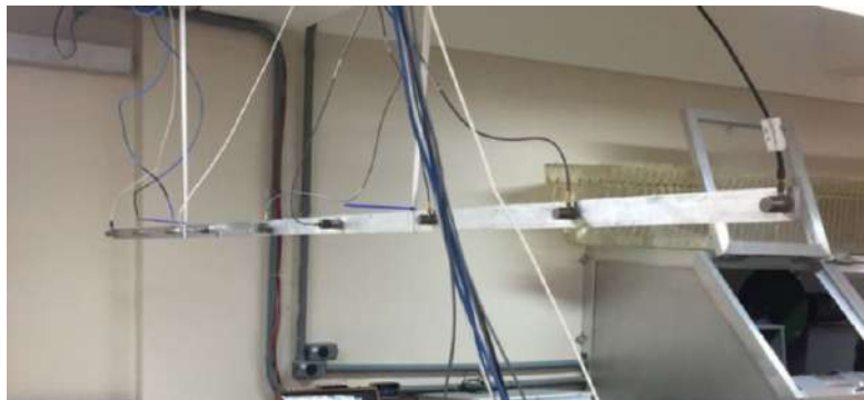
Figure 5.2: Rectangular beam suspended in Free-Free boundary condition and instrumented with 09 accelerometers.
