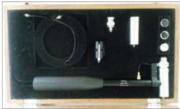
Figure 5.6: Impact Hammer Brüel e Kjaer model 8200.
