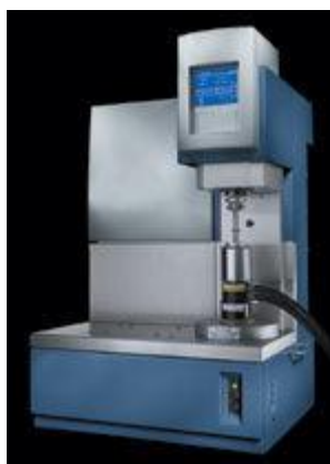
Figura 15: Reômetro ARES® (Advanced Rheometric Expansion System).
