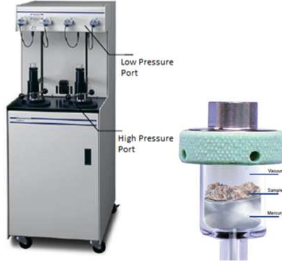
Figure 2.3: AutoPore IV Series Mercury Porosimeter (left) and glass penetrometer (right) used in automated MICP acquisitions.
