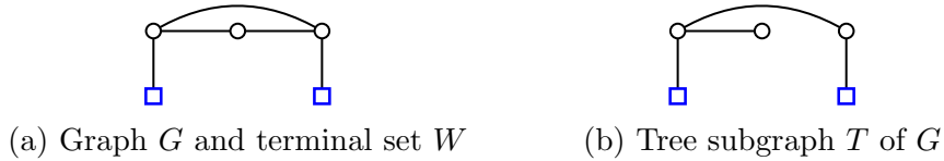
Figure 2.2: (a) A graph G , a terminal set W (blue squares) such that, for every r \geq 0 and for \ell = 1 , (G, W, \ell, r) is a no -instance of TCP, since every connection tree of G for W has at least 2 linkers. (b) A tree subgraph T of G such that W \subseteq V(T) but \text{leaves}(T) \not\subseteq W , which contains exactly one non-terminal vertex of degree 2 and exactly one non-terminal vertex of degree at least 3.
