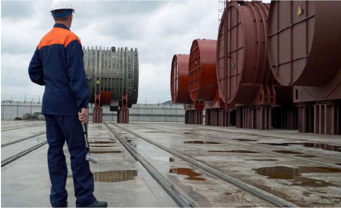
Figure 3 - Reactor compartments on interim repositories at Sayda Bay
