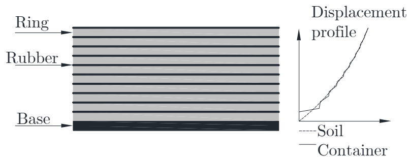
Figure 2.12: Schematic representation of an Equivalent Shear Beam Container (adapted from Bhattacharya et al. , 2012).
