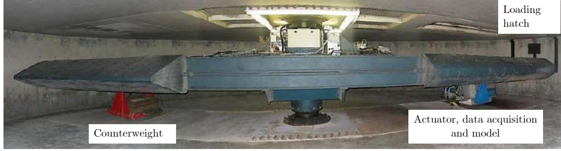
Figure 3.1: A view of the Turner Beam Centrifuge at the Schofield Centre – University of Cambridge.
