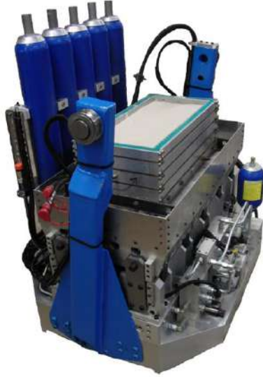
Figure 3.3: Servo-hydraulic earthquake actuator.
