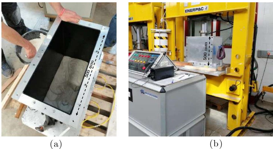
Figure 3.10: a) Pouring of the clay at a water content of 120%; b) Consolidation in a computer-controlled consolidation rig.
