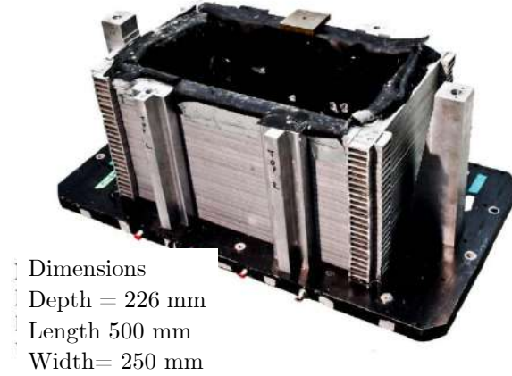
Figure 2.15: A view of the laminar container used at the Schofield Centre, University of Cambridge. .
