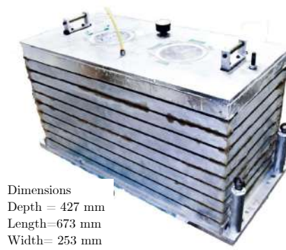
Figure 2.13: Examples of Equivalent Shear Beam containers used in centrifuge testing at the Schofield Centre, University of Cambridge.
