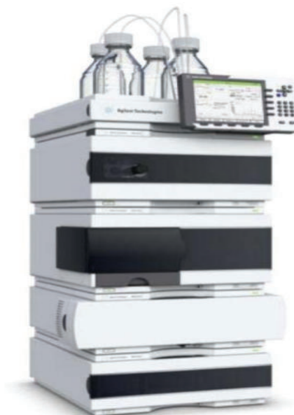
Figura 9 – HPLC Agilent 1260 Infinity.
