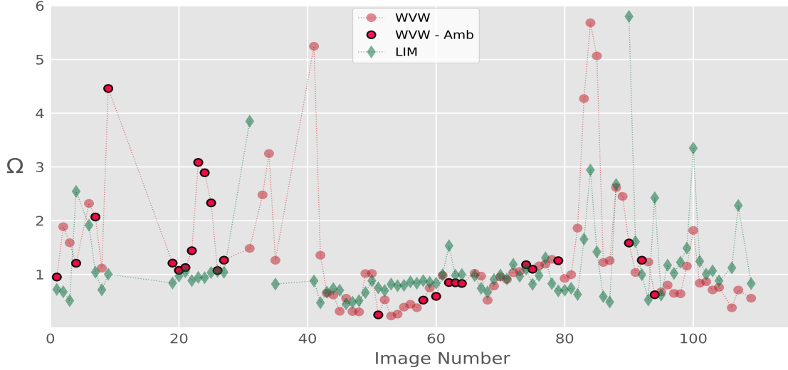
Figure 5.3: The parameter \Omega (Equation 5.1) is a matrix square error normalized with the square of the reference wave spectrum (ERA5), computed along the ground track shown in Figure 5.1. Small values of \Omega indicate close proximity between spectra. For wave spectra retrieved with the LIM (green diamond) and with the ESA procedure (WWV, pink circle). Also shown, as red circles, the cases where the directional ambiguity was not properly resolved (WWV - Amb) — Equation 5.2.
