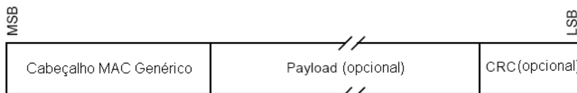
Figura 4.2: Quadro MAC (fonte [1])
