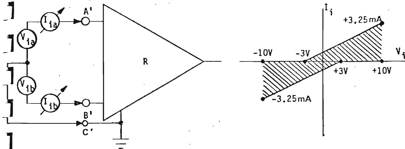
FIGURE 4.4 Receiver Input Current-Voltage Measurement
