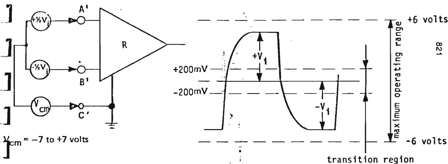
FIGURE 4.5 Receiver Input Sensitivity Measurement
