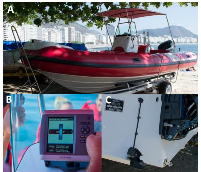
Fig. 6. Cação, the boat hired for the MNIC survey. A: Single hull inflatable construction, general view; B: view of cockpit, with the Garmin GPSMap 521 echosounder; C: hull with a 115 HP engine. Note echosounder transducer near the hull bottom.
