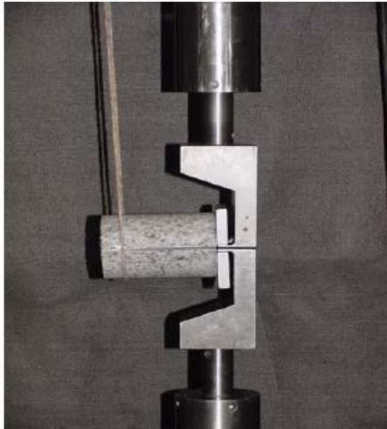
**Figura 4.7** – Ensaio Short Rod (ISRM 1988, *in* Pehovaz-Alvarez et al., 2004).
