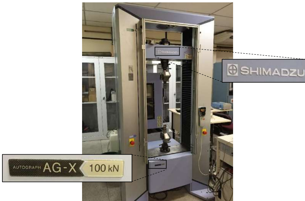
Figure 4.6 – Machine used to perform the test characterization of materials.
