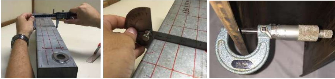
Figure 4.2 – Specimens dimensional manual measurements.
