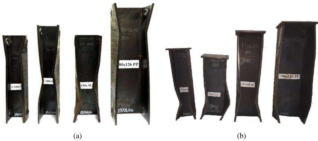
Figure 4.17 – Joint view of the specimens (a) 100x70C- P_F /100x100C- P_F /130x91C- P_F /180x126C- P_F and (b) 100x70C- P_{FF} /130x91C- P_{FF} /150x105C- P_{FF} /180x126C- P_F after the load removal.
