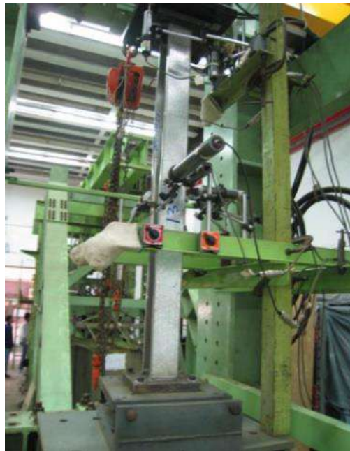
Figure 1.1 – Test in an open section column with rigid plates welded at the ends [26].
