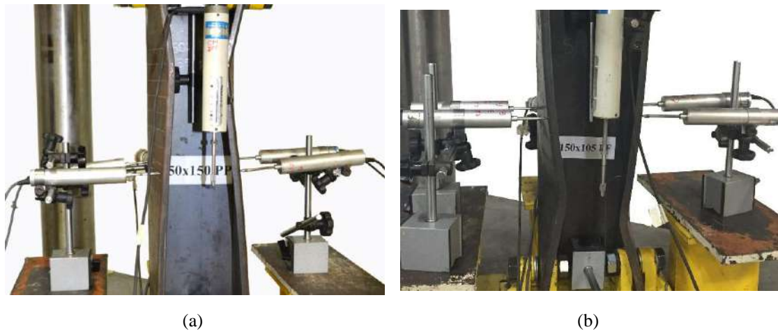
Figure 4.18 – Close view of the most deformed region of specimen (a) 150x150C- P_F and (b) 150x105C- P_{FF} just after collapse.
