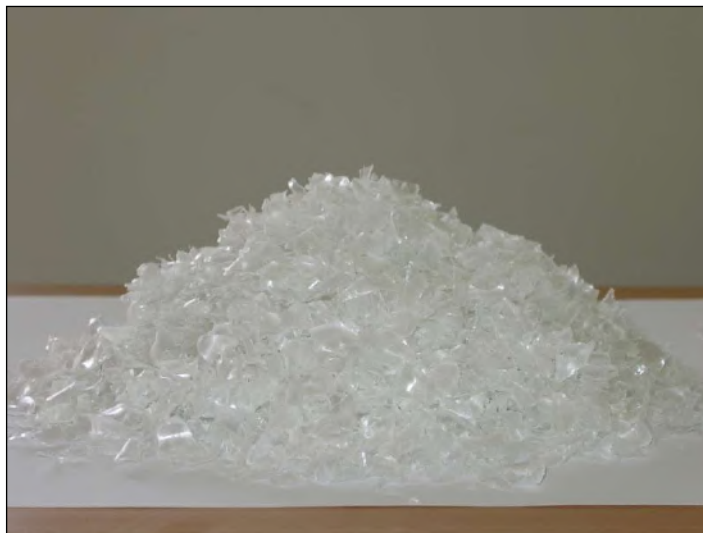
Figura 23 – Flake de PET reciclado (VERTEX TRADE AND TECHNOLOGY S/A, 2009)
