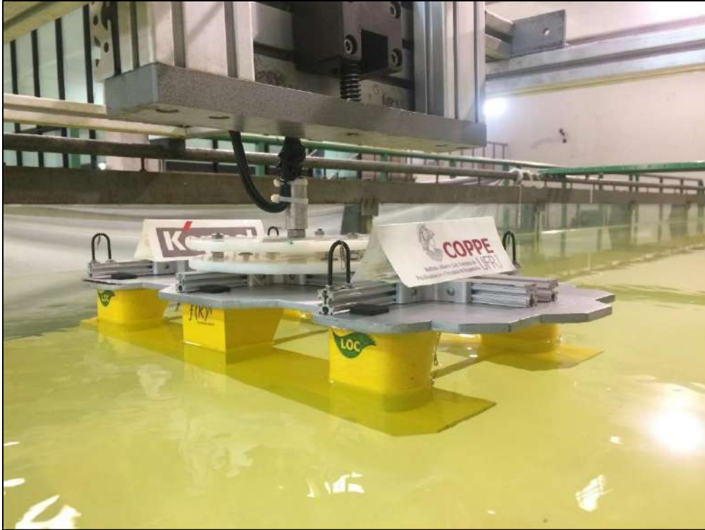
Figure C.4 Current load tests for the TAD in single-body case.
