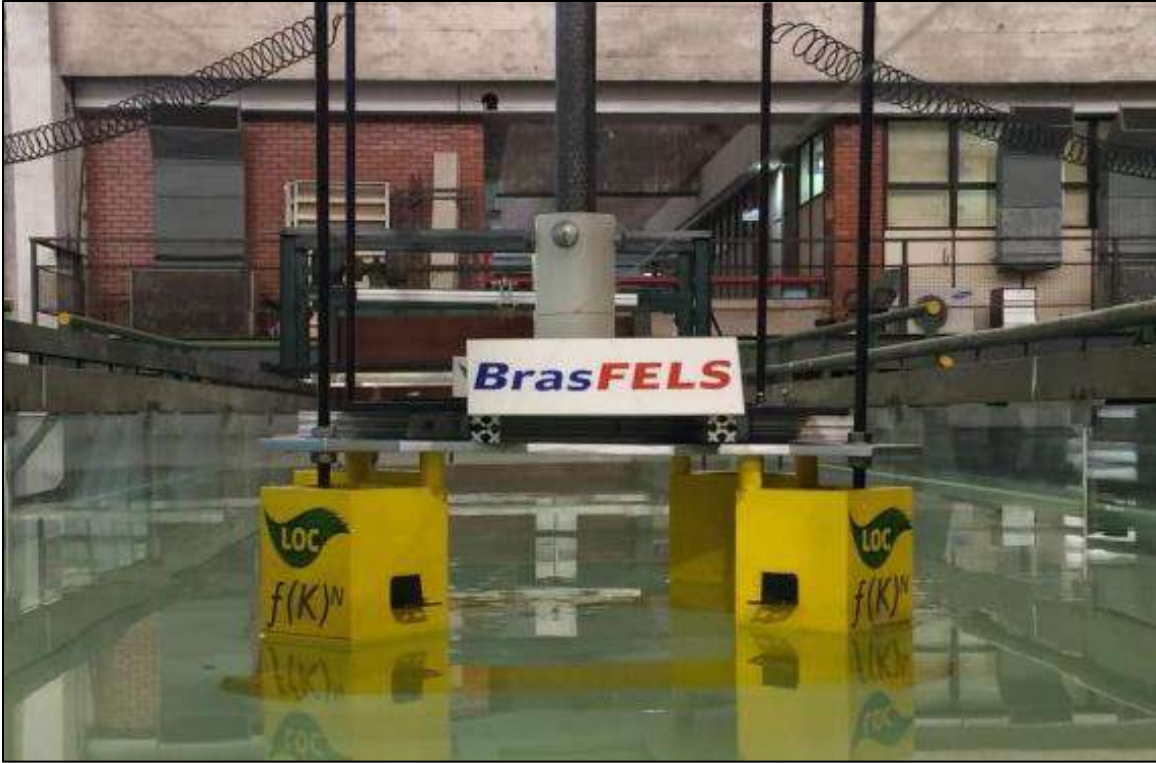
Figure C.6 VIM test of the TLP.
