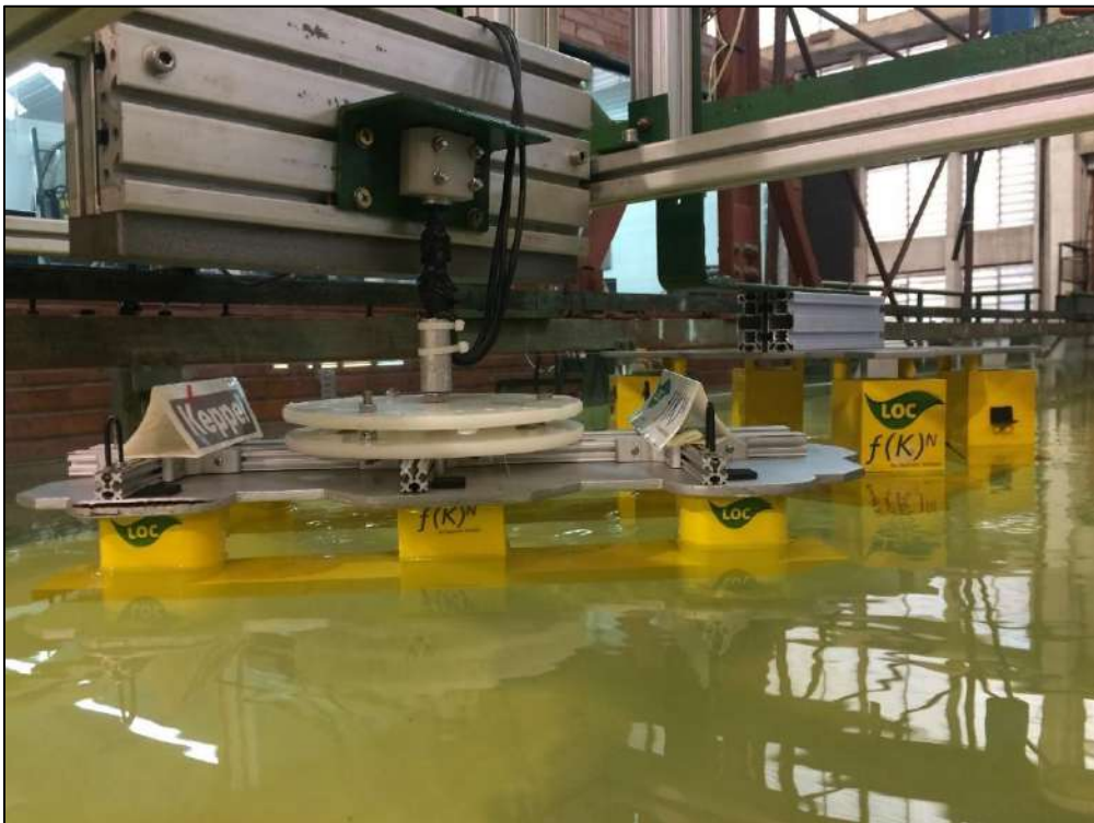
Figure C.5 Current load tests for the TAD Upstream in multi-body case.
