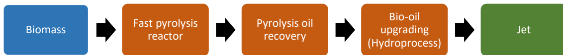
Figure 15: Main steps in the HDCJ process. Based on (ELGOWAINY et al., 2012; GUELL et al., 2012)
