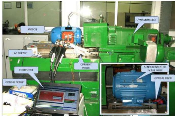
Fig. 10. Experimental setup assembled at Weg workshop. Inset: Induction motor showing the sensor inserted in a hole that penetrated through the stator frame up to the air gap.
