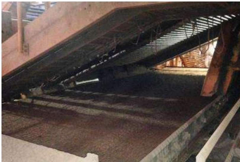
Figure 3.21. Conveyor belt for transport of fines sieved on double deck roller screen at Vargem Grande induration machine entrance.
