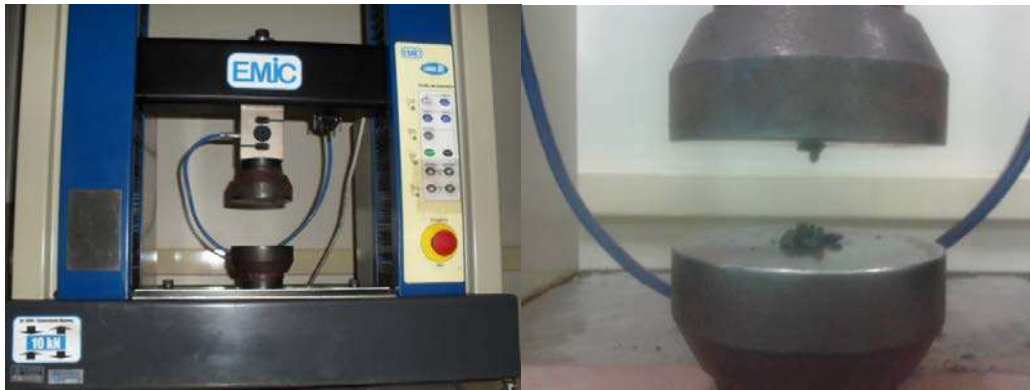
Figure 4.5. Compression test on EMIC 10 kN press.
