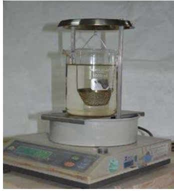
Figure 4.2. Hydrostatic density test setup.
