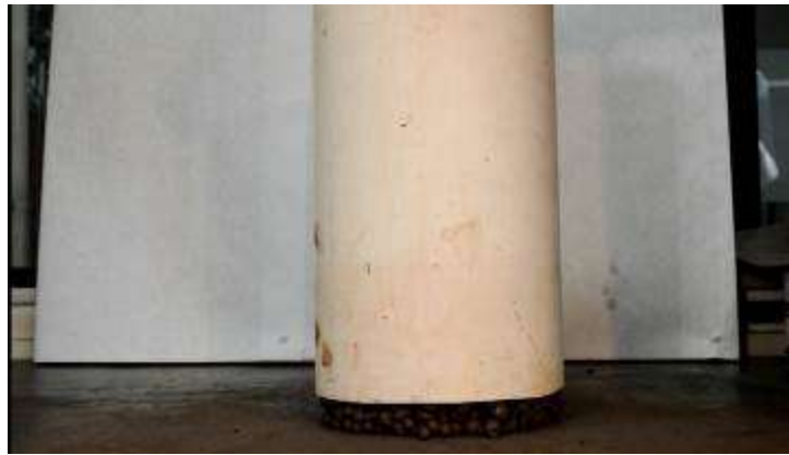
Figure 4.6. Hollow cylinder filled with pellets.
