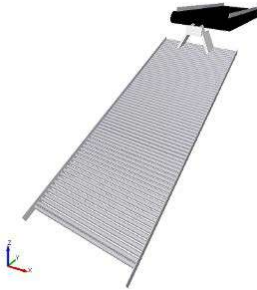
Figure 4.10. Feed conveyor and roller screens in EDEM ® creator platform.
