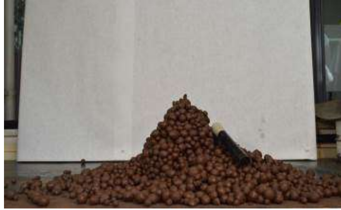
Figure 5.4. Repose angle test: final pile disposal profile.
