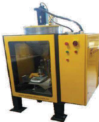
Figura V.2 – IDEA - Impact Degradation Energy Analyzer.
