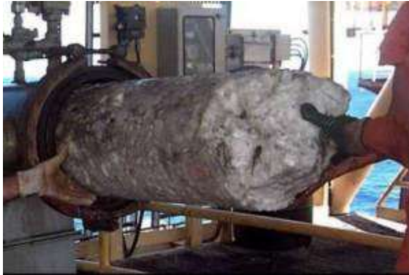
Figure 2-5 Hydrate plug removed from a flowline (Photograph courtesy of Petrobras)
