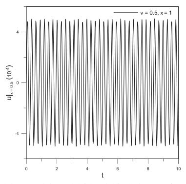
**Fig. 9.** Dimensionless transverse displacement u(x,t) of a clamped axially moving beam at x = 0.5 for v = 0.5 and  $\zeta = 1$ .
