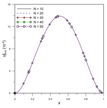
**Fig. 1.** GITT solutions with different truncation orders *N* for the dimensionless transverse displacement u(x,t) of a clamped axially moving beam at t = 5 for v = 0.15 and  $\xi = 0.1$ .
