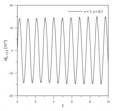
**Fig. 6.** Dimensionless transverse displacement u(x,t) of a clamped axially moving beam at x = 0.5 for v = 1 and  $\xi = 0.1$ .
