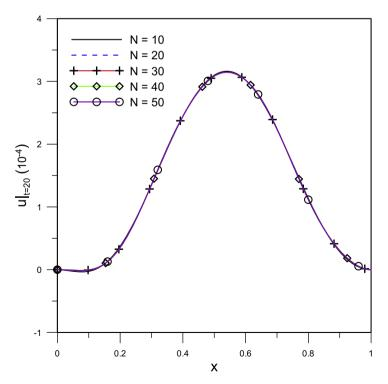
**Fig. 2.** GITT solutions with different truncation orders *N* for the dimensionless transverse displacement u(x,t) of a clamped axially moving beam at t = 20 for v = 0.15 and  $\xi = 0.1$ .
