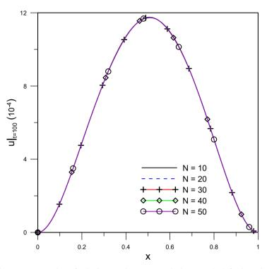
**Fig. 3.** GITT solutions with different truncation orders *N* for the dimensionless transverse displacement u(x,t) of a clamped axially moving beam at t = 100 for v = 0.15 and  $\xi = 0.1$ .
