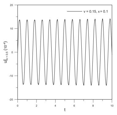
**Fig. 5.** Dimensionless transverse displacement u(x,t) of a clamped axially moving beam at x = 0.5 for v = 0.15 and  $\zeta = 0.1$ .
