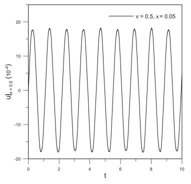
**Fig. 7.** Dimensionless transverse displacement u(x,t) of a clamped axially moving beam at x = 0.5 for v = 0.5 and  $\zeta = 0.05$ .
