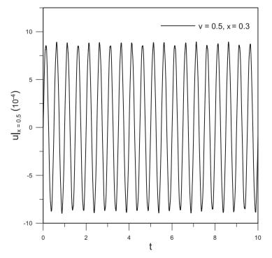
**Fig. 8.** Dimensionless transverse displacement u(x,t) of a clamped axially moving beam at x = 0.5 for v = 0.5 and  $\xi = 0.3$ .
