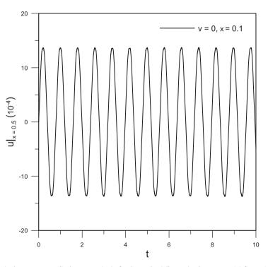
**Fig. 4.** Dimensionless transverse displacement u(x,t) of a clamped axially moving beam at x = 0.5 for v = 0 and  $\xi = 0.1$ .
