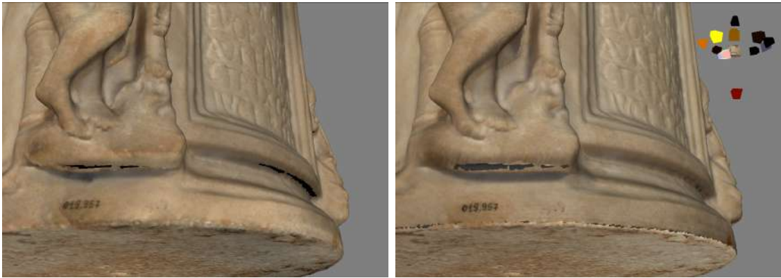
Figure 5.7: Traditional texture mapping (left) and proposed method (right). Note the sharper numbers at the base of the urn with our method.
