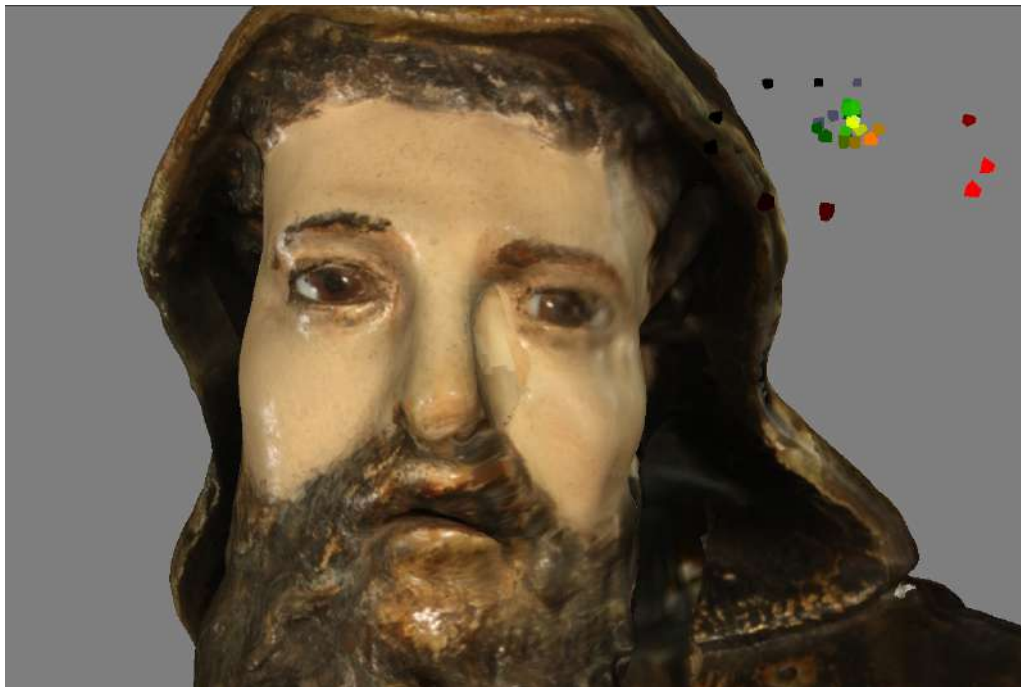
Figure 5.3: In a close-up view, weights are given for the photos taken from near the object or with zoom. Note, however, that the left side of the face was better sampled than the right, causing some artifacts on the right side.
