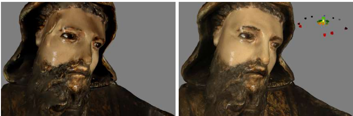
Figure 5.6: Traditional texture mapping (left) and our proposed method (right). Note how our method produces a much sharper visualization since only a few images have significant weight for the view position.
