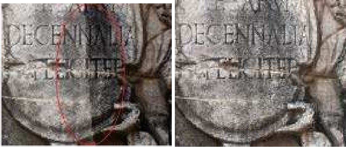
Figure 2.3: Color and brightness correction to remove seams. Texture model without correction (left) and with correction (right). Images extracted from PREVITALI et al. [2].
