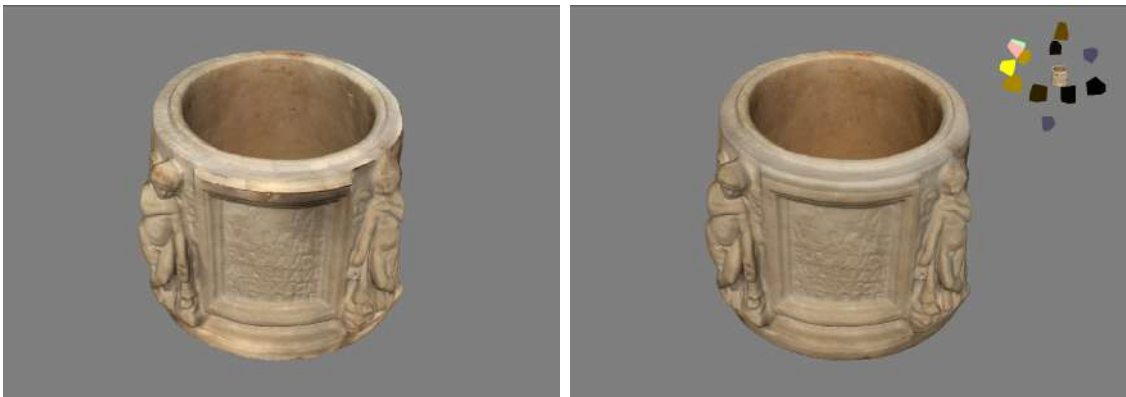
Figure 5.9: Traditional texture mapping(left) and proposed method (right). Illumination variations are better handled with our method, since oblique cameras receive very low weights. Note that artifacts are visible near borders in traditional texture mapping
