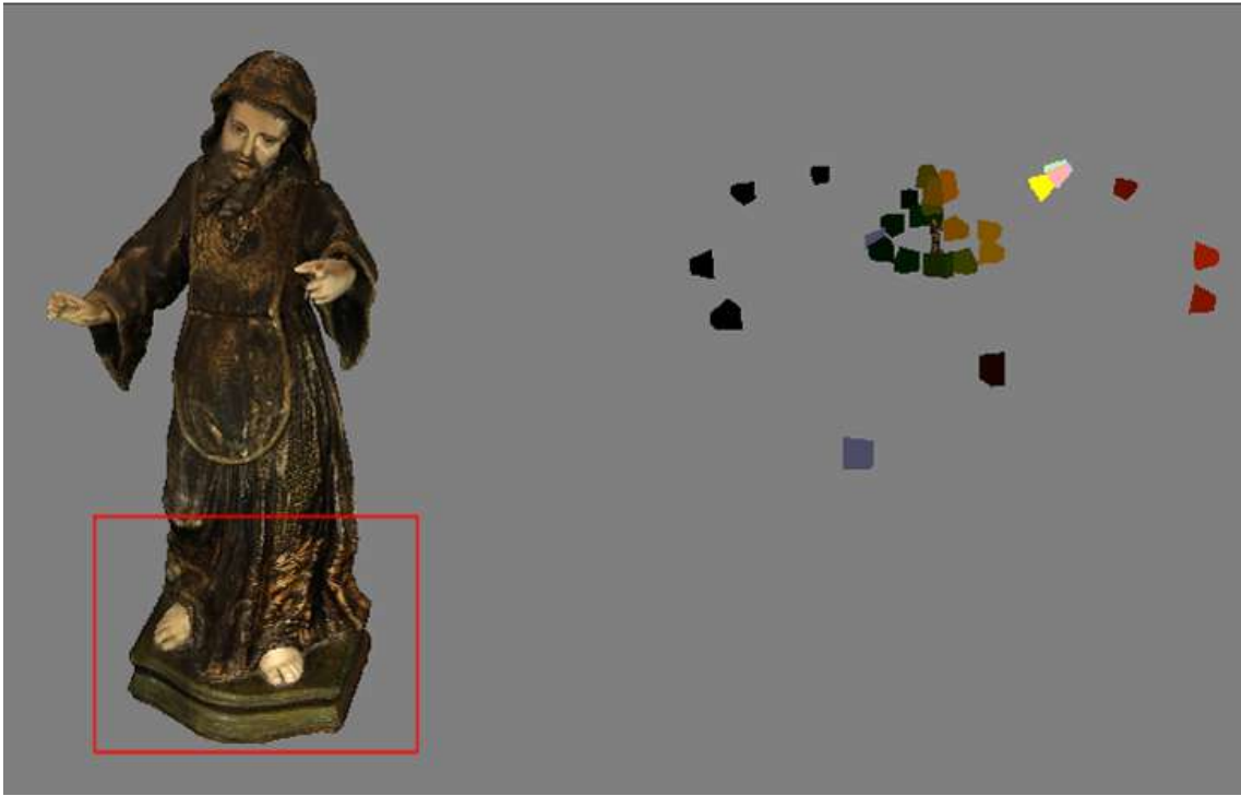
(a) The red box shows a region where the color projection was improved after normalizing the FOV for all cameras. On the right are shown the cameras in respect to the model.
