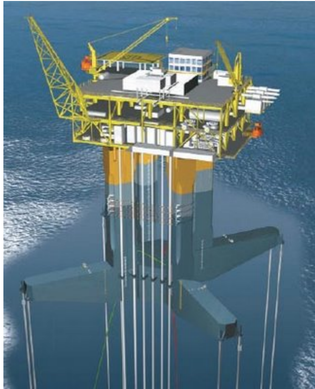
Figura 4.11 - TLP. Fonte: Oil and Gas Processing
