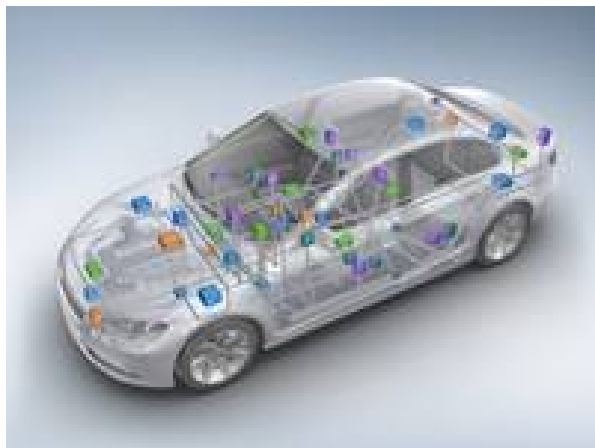
Figure 1.1: ECUs in a modern vehicle.
