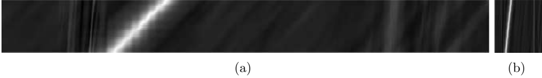
Figure 3.12: Example of resulting \mathbf{W}_t matrices from Eq. (3.1) using: (a) complete reference data matrix \mathbf{X}_r ; (b) downsampled-in-time reference matrix \mathbf{X}_r^{\text{ds}} .
