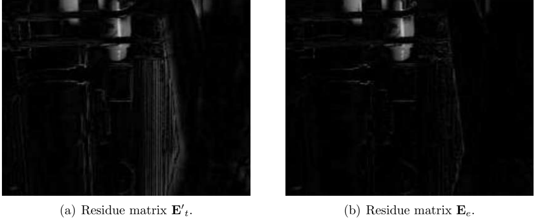
Figure 3.10: There are fewer undesired artifacts in the residue matrix \mathbf{E}_e when compared with \mathbf{E}'_t .
