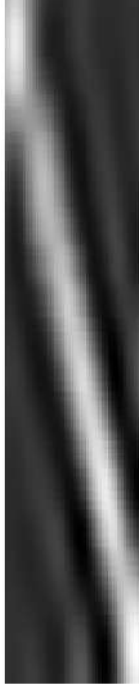
Figure 3.1: Matrix \mathbf{W}_t generated with mcRoSuRe method. Brighter pixels denote higher values in the matrix. The horizontal dimension corresponds to the target video frames and the vertical dimension to the reference video frames. The region from which the frames from the reference video were taken to reconstruct the target frames can be seen here.
