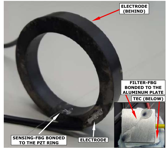
Fig. 7. Sensing-FBG bonded to the inner diameter of a ring-shaped PZT ceramics. Inset: filter-FBG bonded to the surface of an aluminum substrate.
