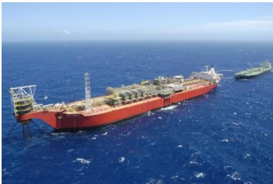
*Figura 2.8 –Turret Externo do FPSO Fluminense.*
