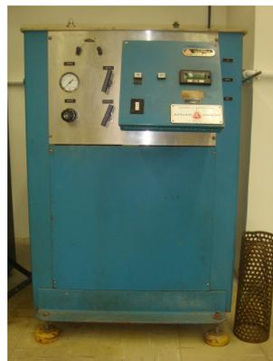
**Figura 3.9:** Prensa Isostática Autoclave Engineers Eries, P.A.
