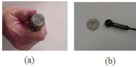
Figure 4.1: (a) multicomponent sensor and (b) spherical source.
