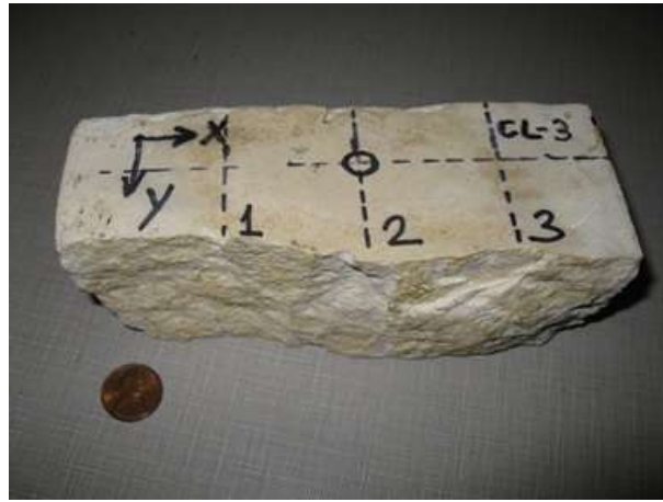
Figure 4.2: Carbonate sample for rock properties study.
