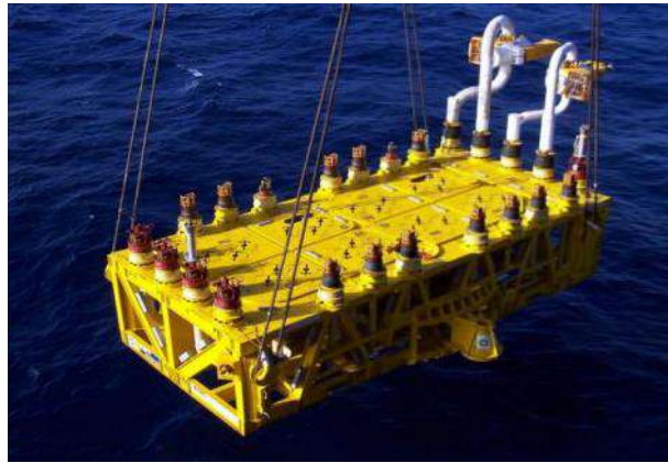
Figura 2.8 Cluster manifold com 10 slots (WANG et al, 2012)
