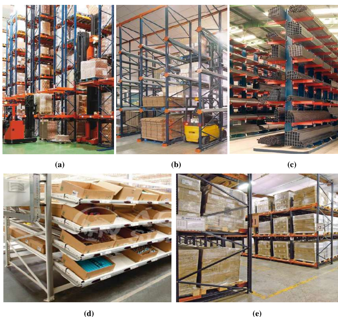
Figura 1.5. Estruturas (a) porta-pallets , (b) drive-in , drive-through , (c) cantilever , (MECALUX,2016) 2 (d) flow-rack (ÁGUIA SISTEMAS, 2016) 4 e (e) push-back (MECALUX, 2016) 2 .
