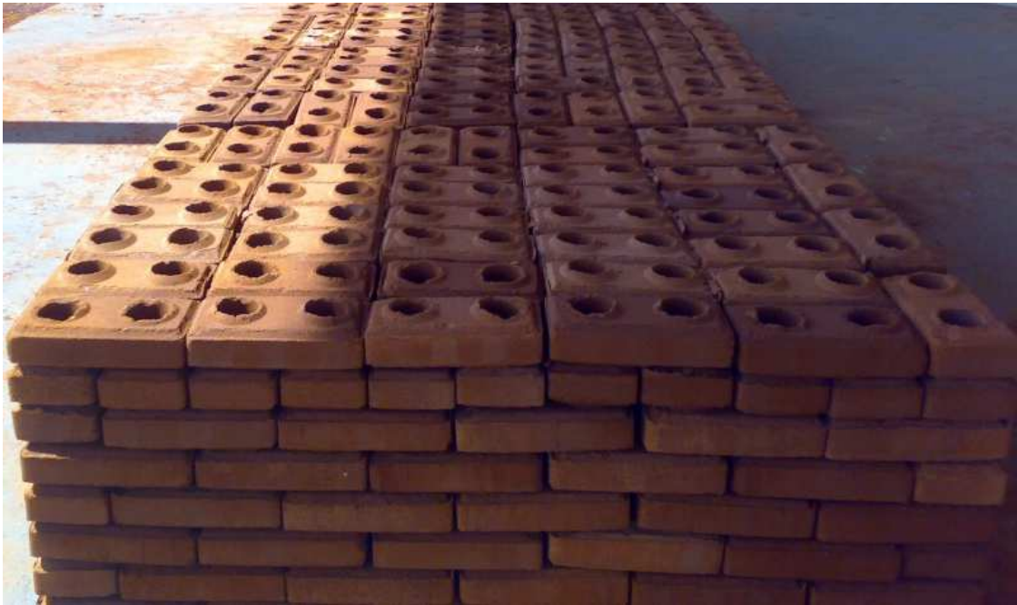
Figura 2-4 Tijolo de solo-cimento (Wordpress 2011)
