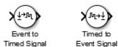
Figure 3.8: Signal converters: the time to event signal, on the left, and the event to timed signal, on the right
