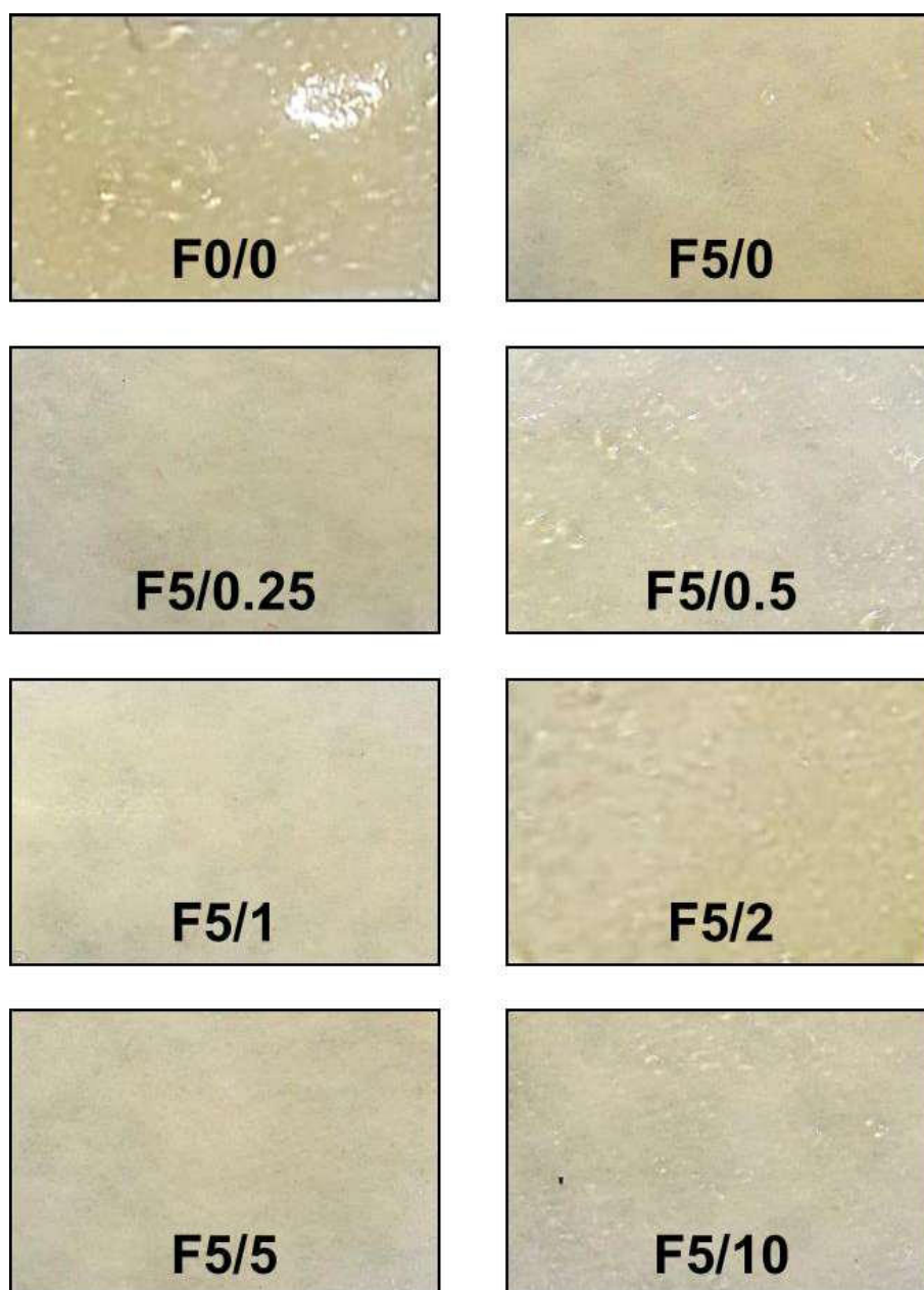
Figure 62. Digital pictures of the CS-DES-based films. F0/0: 0% DES and 0% açai PECs; F5/0: 5% DES and 0% açai PECs; F5/0.25: 5% DES and 0.25% açai PECs; F5/0.5: 5% DES and 0.5% açai PECs; F5/1: 5% DES and 1% açai PECs; F5/2: 5% DES and 2% açai PECs; F5/5: 5% DES and 5% açai PECs and F5/10: 5% DES and 10% açai PECs.
